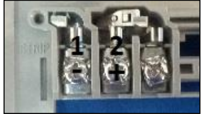
Strobe Wiring Terminals
